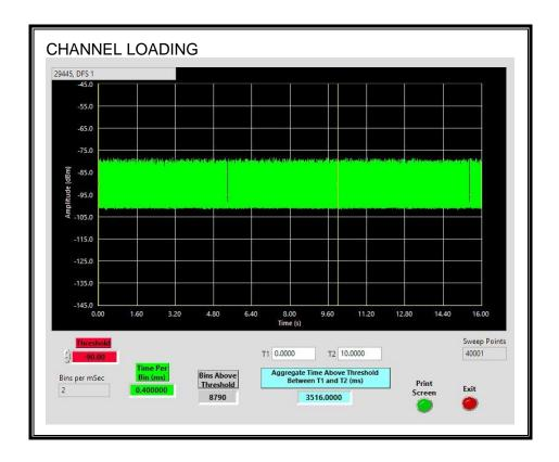
The level of traffic loading on the channel by the EUT is 35.16%
