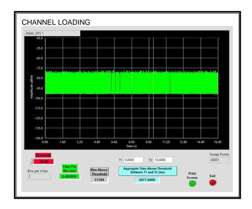
The level of traffic loading on the channel by the EUT is 44.77%
