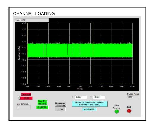
The level of traffic loading on the channel by the EUT is 45.12%
