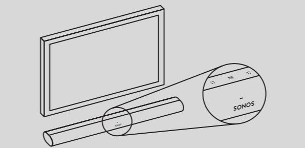
**NOTE:** Make sure the touch controls on Arc are facing up when you position it.
