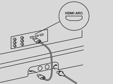
**NOTE:** The optical adapter in the box (optional) is only needed if your TV doesn't have an ARC port. (*Dolby Atmos won't be supported.*)
