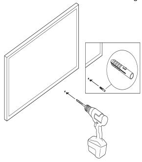
3. If you're using the included wall anchors, use a 5/16" drill bit to drill the pilot holes and then insert the wall anchors. Don't use the anchors if you're drilling into wood or plastic.
