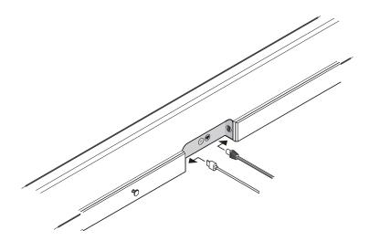
6. Connect the power and HDMI cables to the back of the soundbar.
