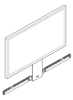
1. If your TV is wall-mounted, place the positioning guide against the wall, aligning the top edge with the bottom of your TV. There should be 4" between the top of the guide and the TV.
