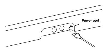
2. Plug the other end of the power cord into an AC (mains) power source.
