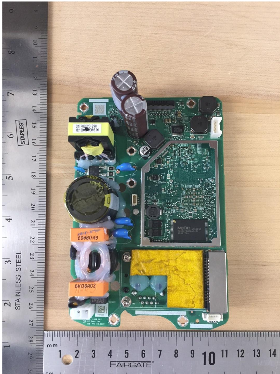
Main board removed RF card Front View
