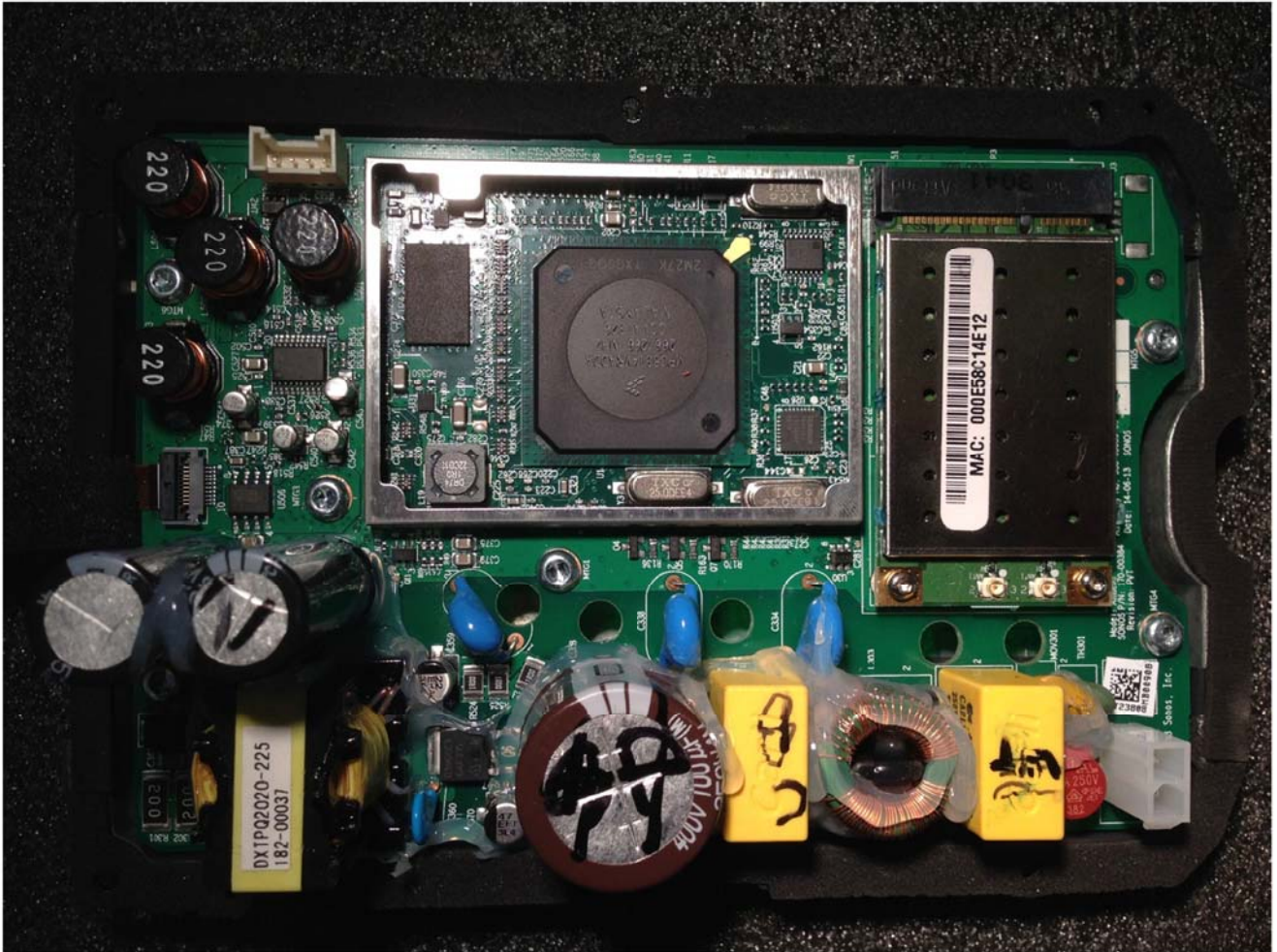
Main PCB top side with radio card
