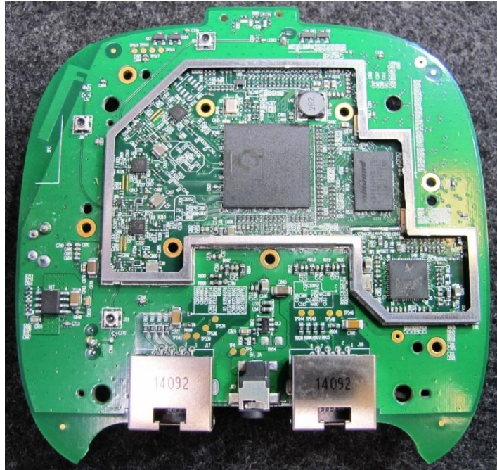
Main PCB bottom without shield
