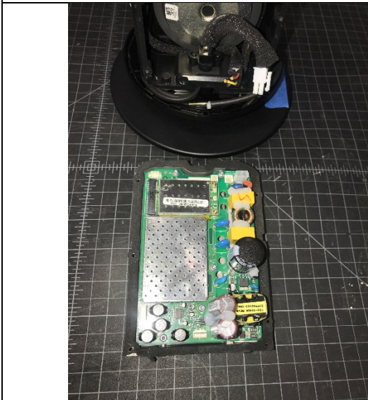
Back Internal PCB on Heatsink
