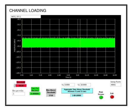
The level of traffic loading on the channel by the EUT is 14.84%
