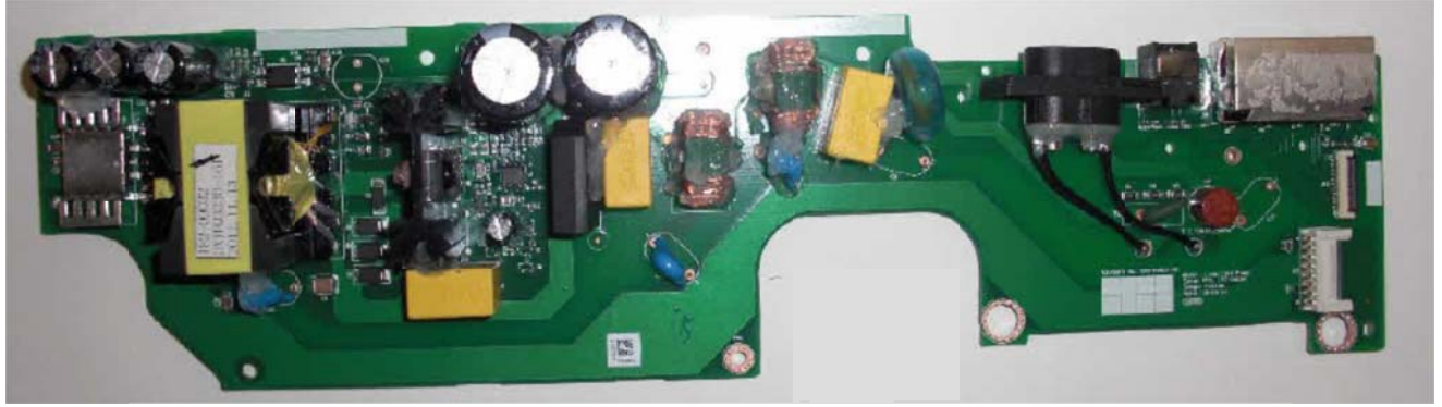
Power Supply Side 1
