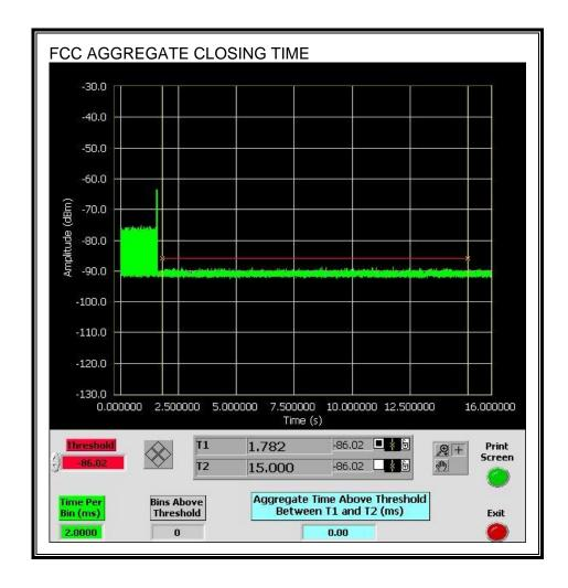
No intermittent transmissions are observed during the IC aggregate monitoring period.
