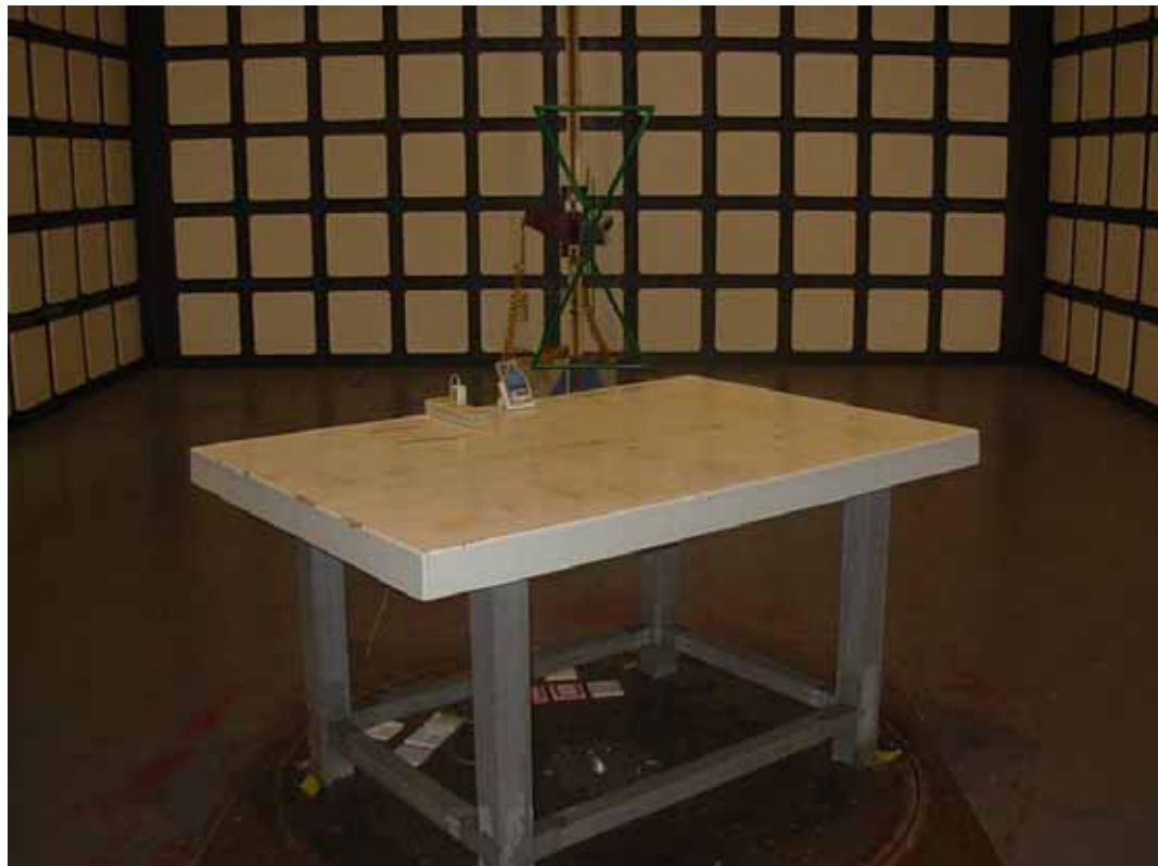
SETUP WITH MAXIMUM DETECTED EMISSION AT VERTICAL POLARIZATION (TRANSMITTING ANTENNA1 CH01)
