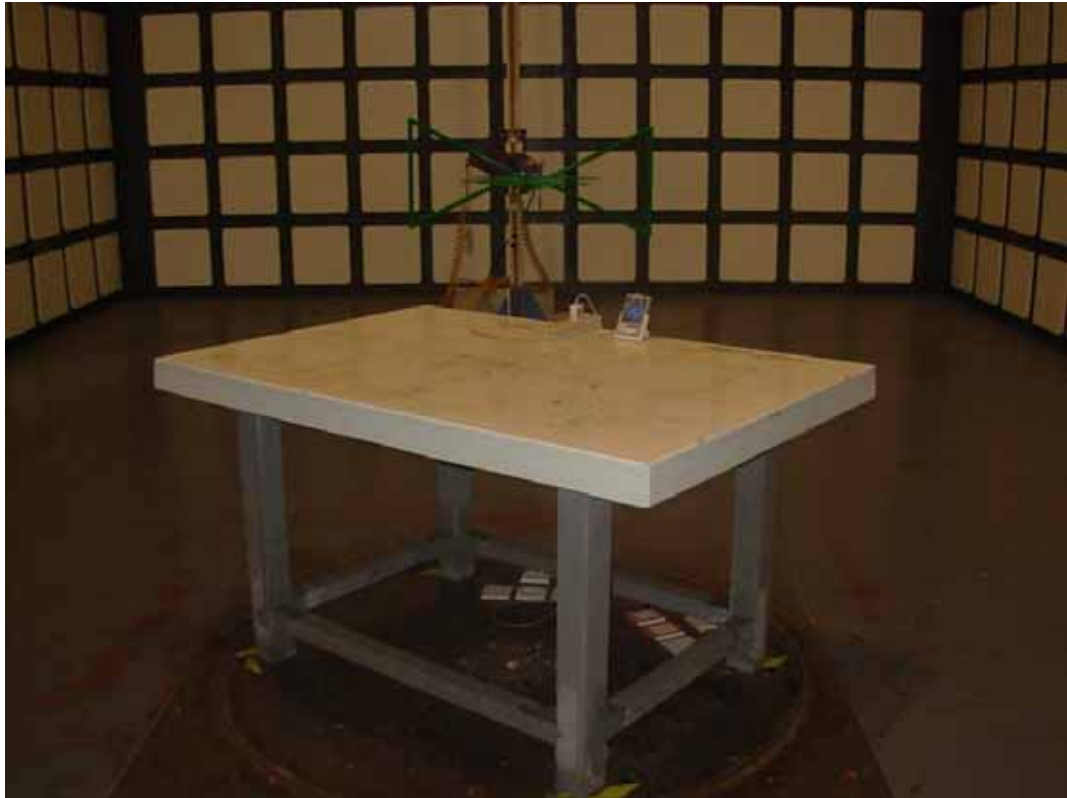
SETUP WITH MAXIMUM DETECTED EMISSION AT HORIZONTAL POLARIZATION (TRANSMITTING ANTENNA1 CH01)
