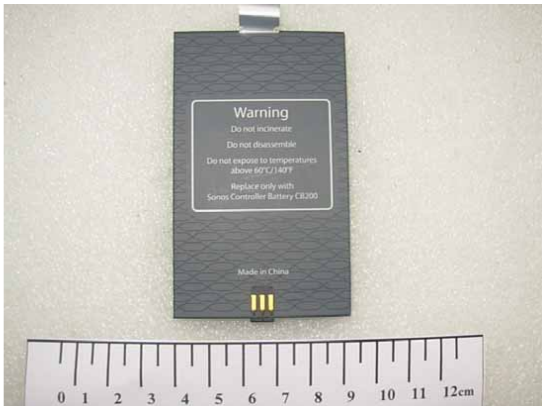
FIGURE 3 WOODSTOCK SONOS CONTROLLER (M/N: CR200) BATTERY BACK
