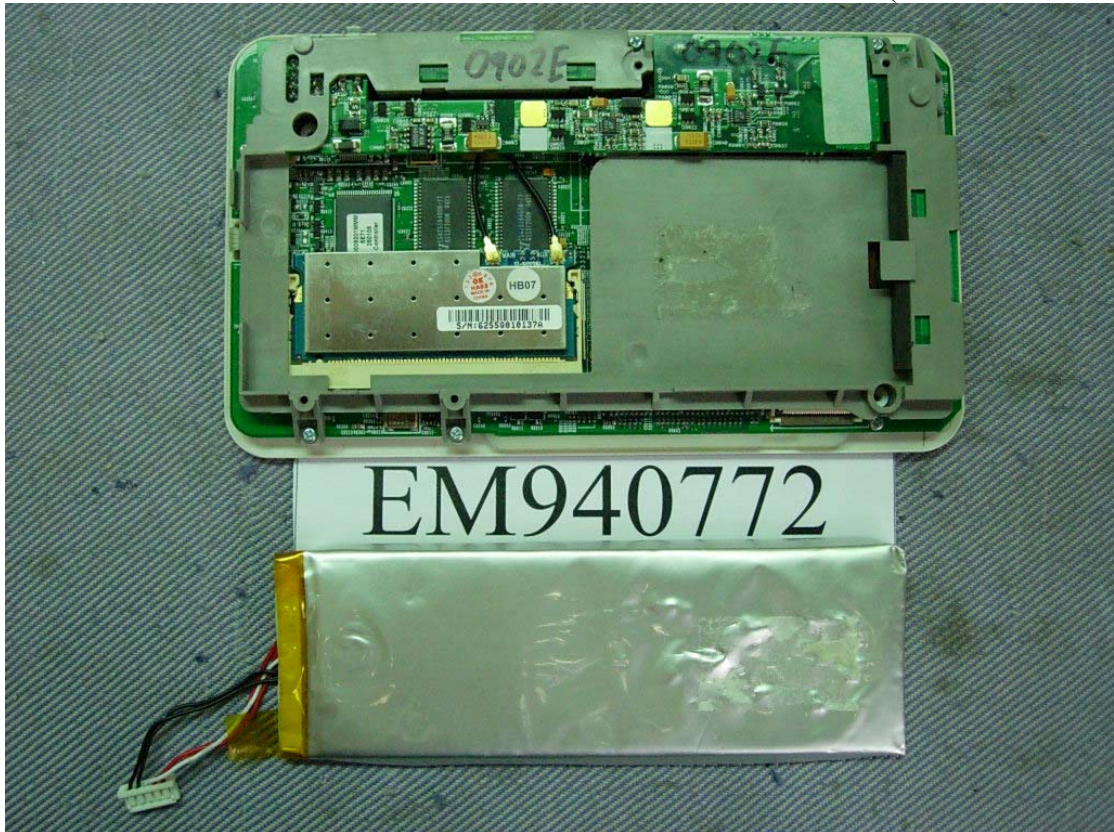
Figure 5 Internal View (Removed Battery)
