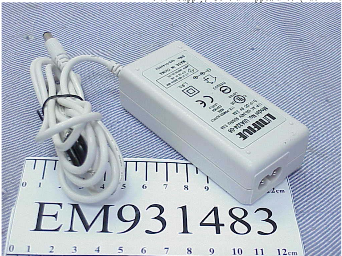
Figure 20 ITE Power Supply, General Appearance (Back View)
