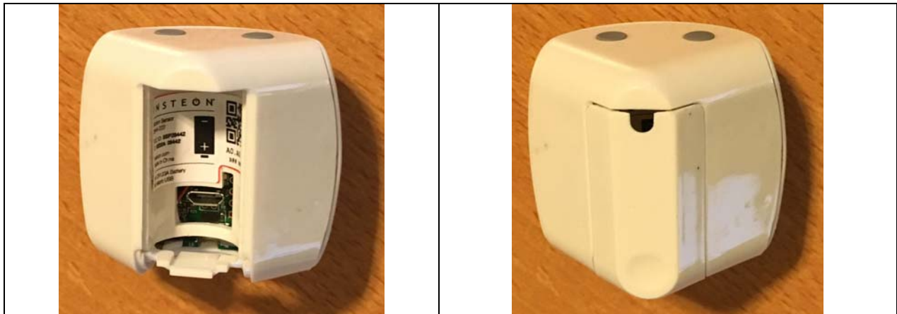
Label placed inside battery compartment
