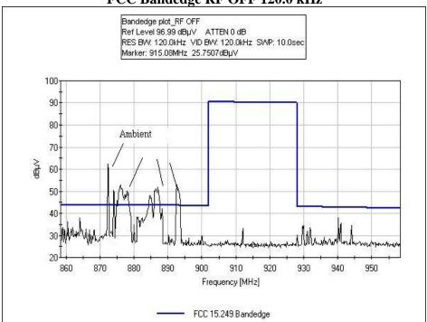
Note: Two plots are presented to clarify the presence of ambient signal; one plot with the Device turned on, the other with the device turned off. The captured Ambient signal is annotated on the plots.
