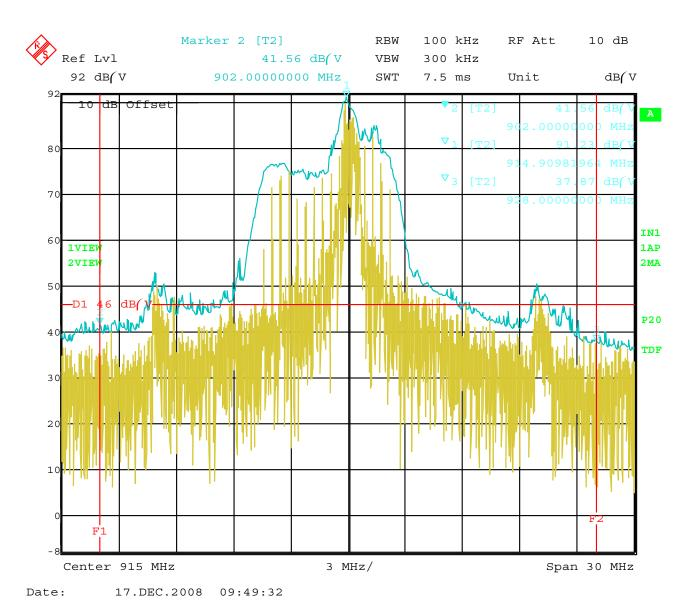
$Band\ Edge\ of\ the\ Fundamental-Z-Axis-Horizontal\ Polarization\ (Worst\ Case)$
