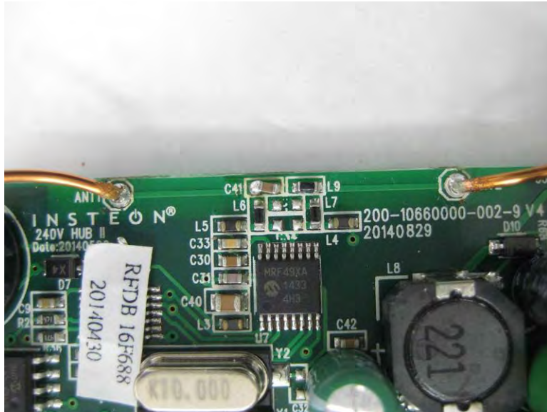
Capacitor C41 (Photo taken by CKC Laboratories)
