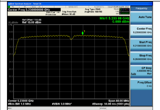
Test Mode:802.11ac VHT40 5230MHz Chain1
