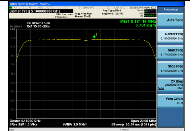
Test Mode:802.11ac VHT20 5180MHz Chain1
