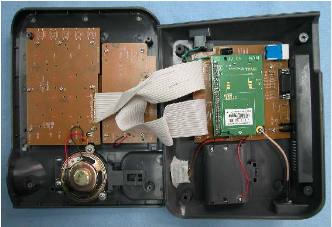
Fixed Wireless Phone Disassembly
