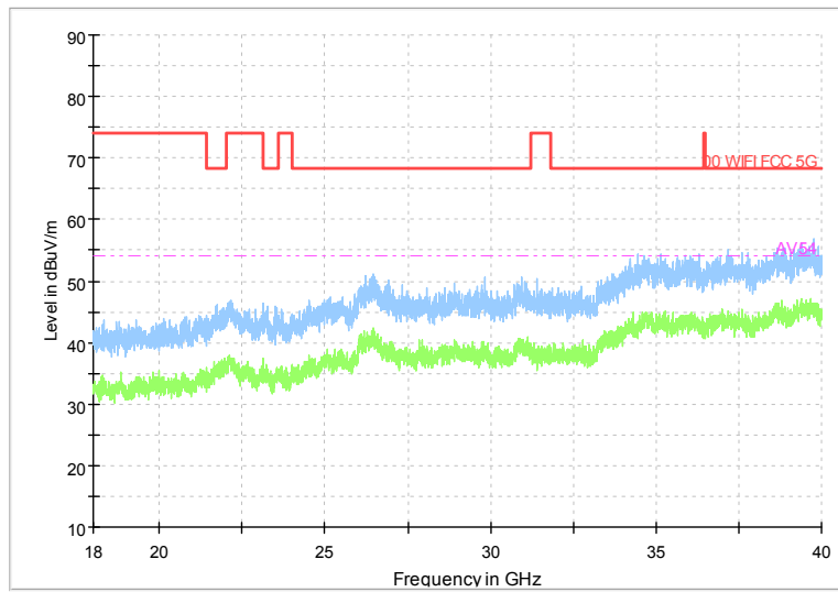
Frequency Range: 18GHz -40GHz Detector: Av mode and PK mode Test Mode: 802.11ax(HE20)
