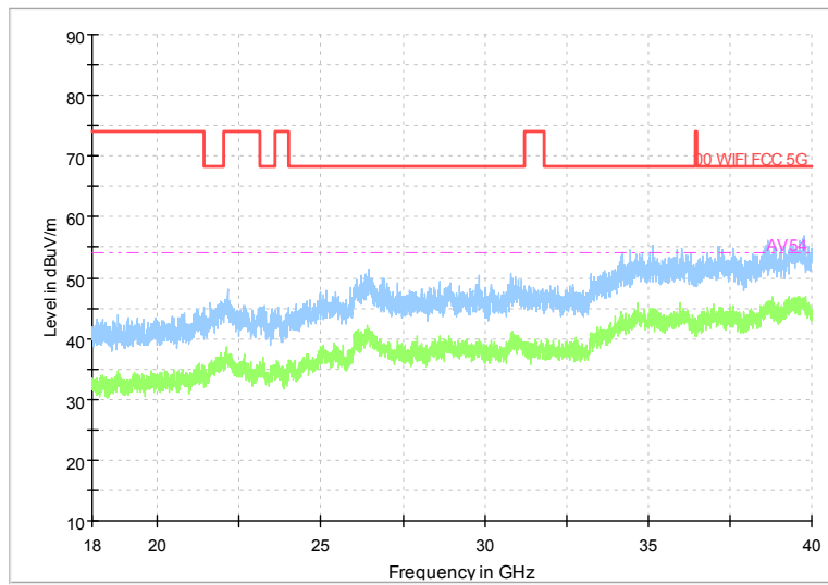
Frequency Range: 18GHz -40GHz Detector: Av mode and PK mode Test Mode: 802.11ax(HE40)
