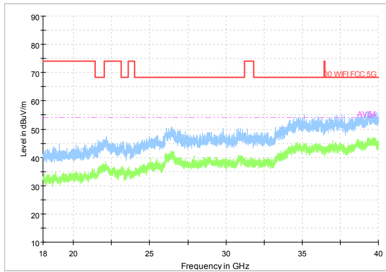
Frequency Range: 18GHz -40GHz Detector: Av mode and PK mode Modulation type: 802.11a
