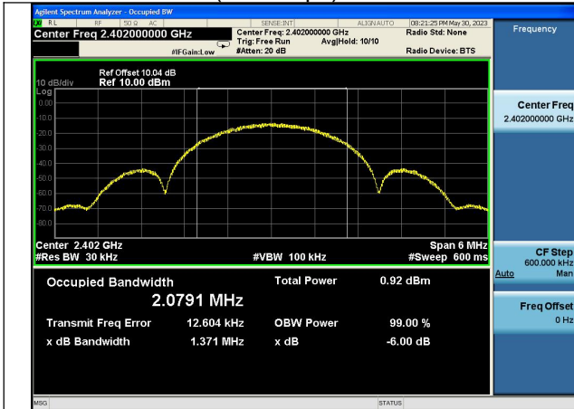
Test Mode:GFSK (LE 2Mbps) 2402MHz
