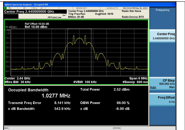
Test Mode:Coded 125K 2440MHz
