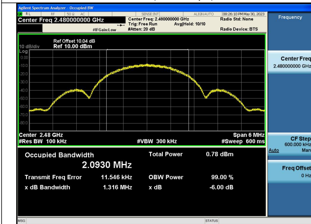
Test Mode:GFSK (LE 2Mbps) 2480MHz
