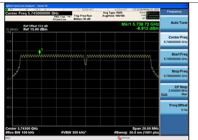
Test Mode:802.11ac VHT20 5745MHz Chain1
