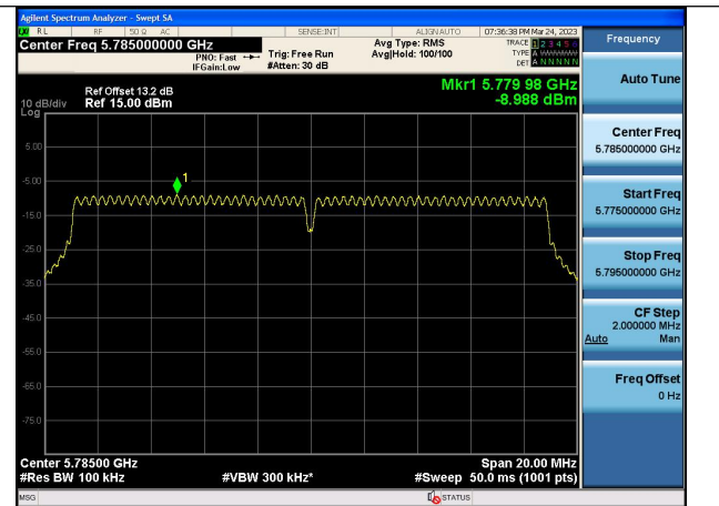
Test Mode:802.11ac VHT20 5785MHz Chain0
