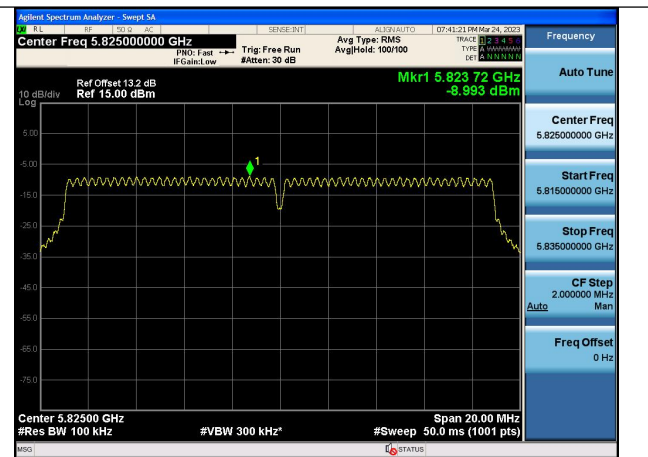
Test Mode:802.11ac VHT20 5825MHz Chain1
