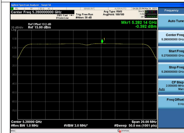
Test Mode:802.11ac VHT20 5280MHz Chain1
