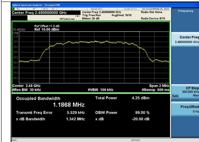
Test Mode: \pi/4 DQPSK(2DH5) 2480MHz
