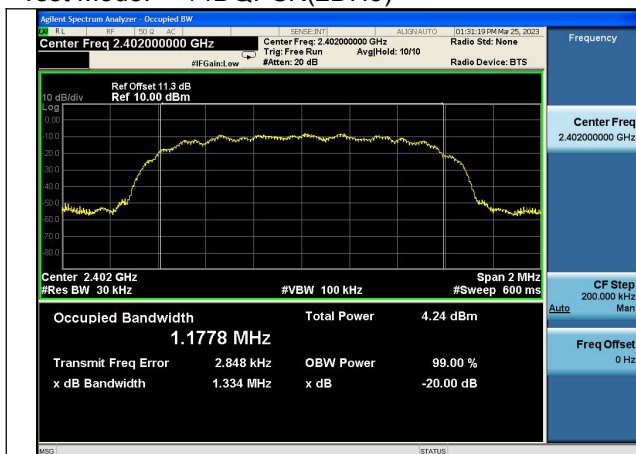
Test Mode: \pi/4 DQPSK(2DH5) 2402MHz
