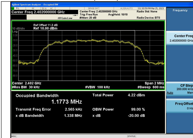
Test Mode: \pi/4 DQPSK(2DH5) 2402MHz
