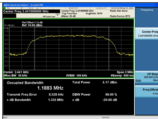
Test Mode:8DPSK(3DH5) 2441MHz
