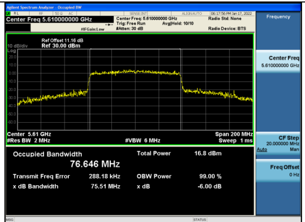
Test Mode:802.11ac VHT80 5610MHz Chain0
