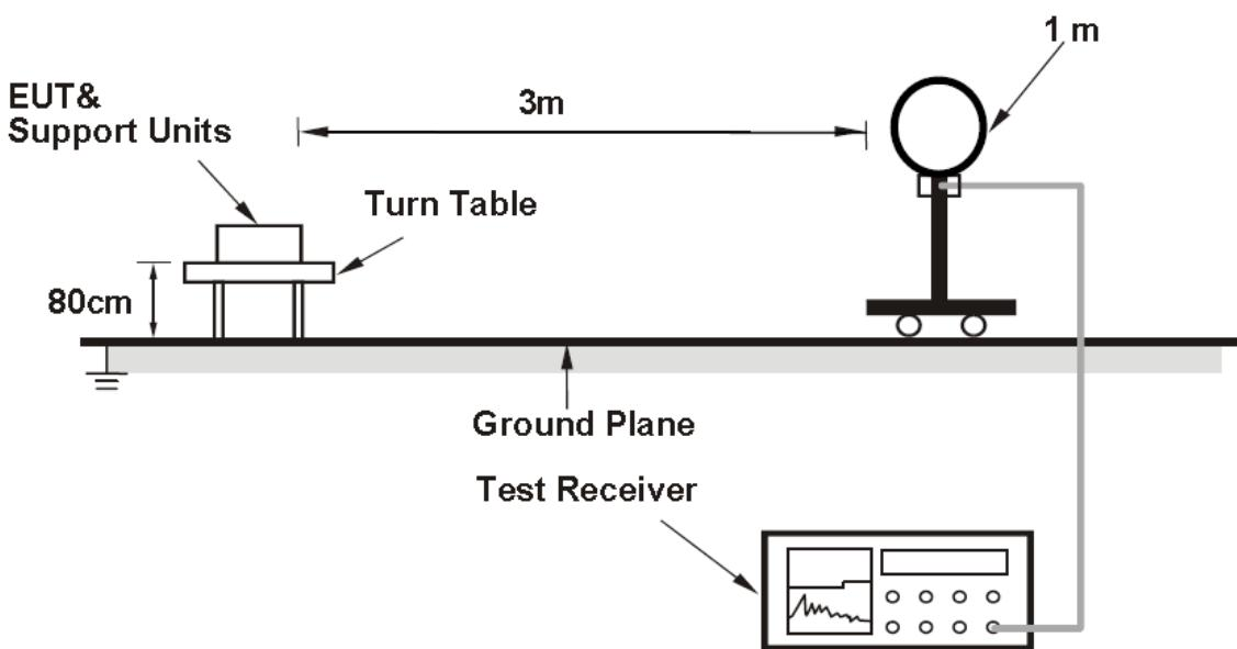
**For Radiated emission 30MHz to 1GHz**
