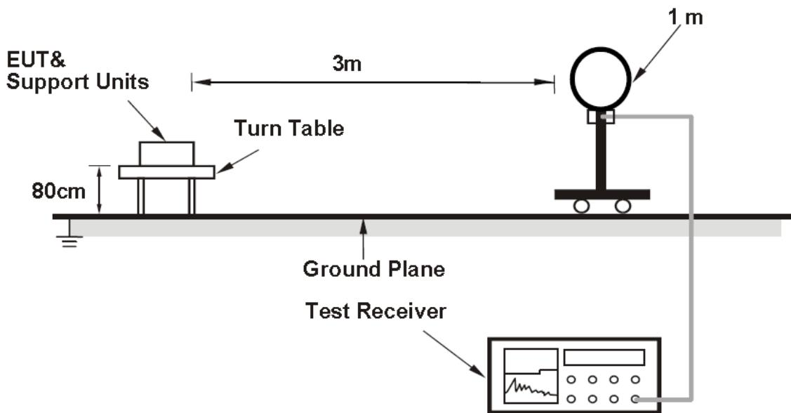
**For Radiated emission 30MHz to 1GHz**
