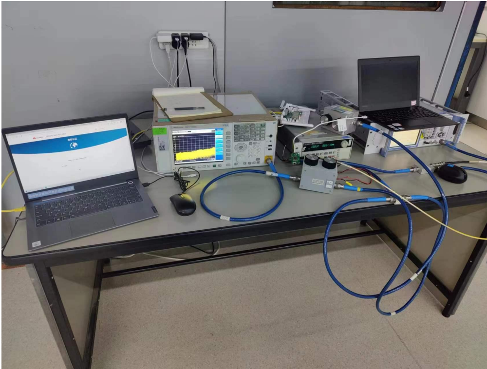
RF Conducted Test setup (BT/WIFI)
