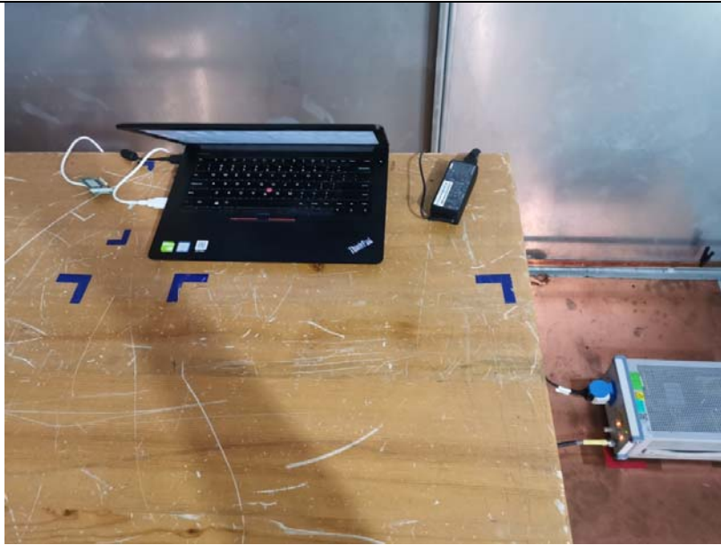
Conducted Emissions Test Setup (with charger)
