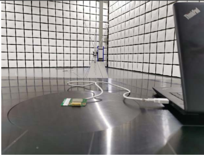
Spurious Radiated Emissions Test setup
