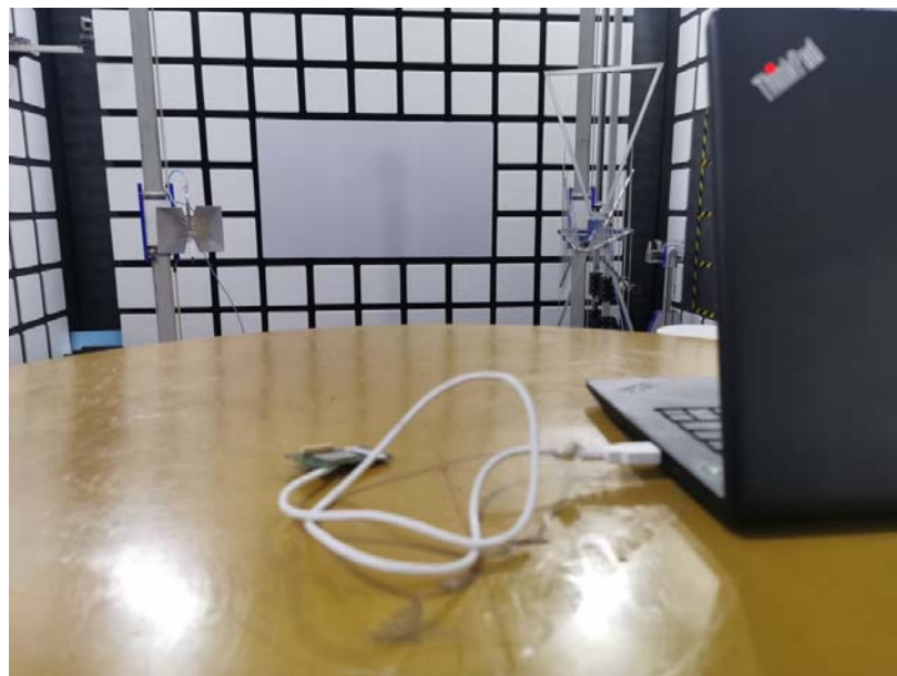
Spurious Radiated Emissions Test setup
