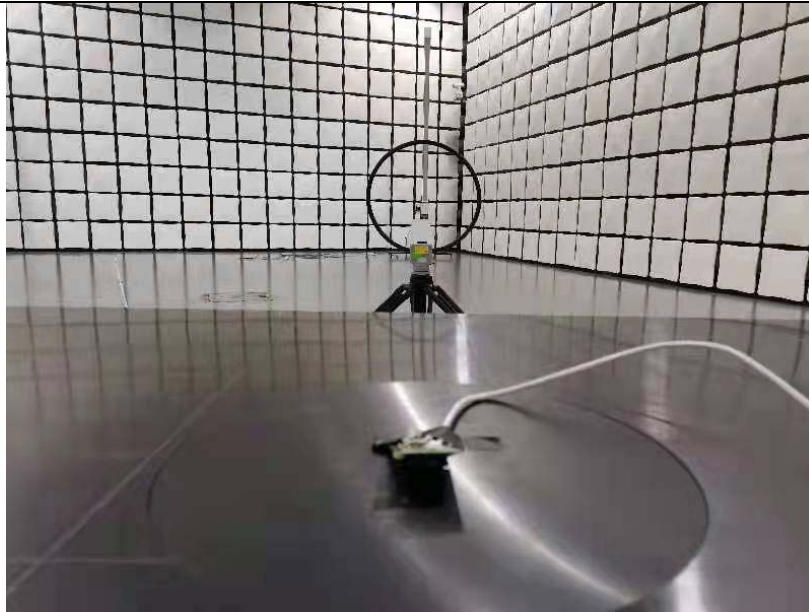
Spurious Radiated Emissions Test setup
