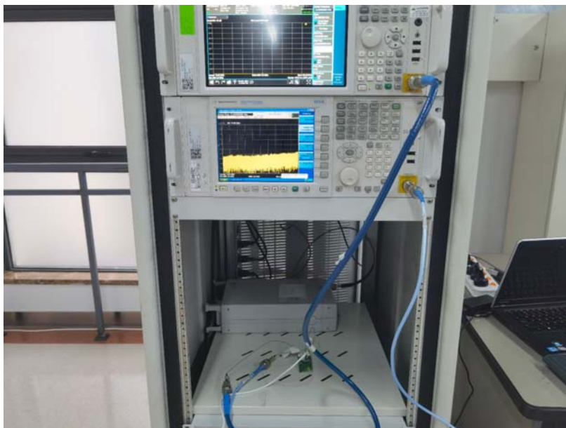
RF Conducted Test setup (BT/WIFI)
