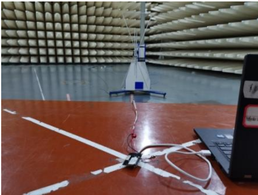
Spurious Radiated Emissions Test setup
