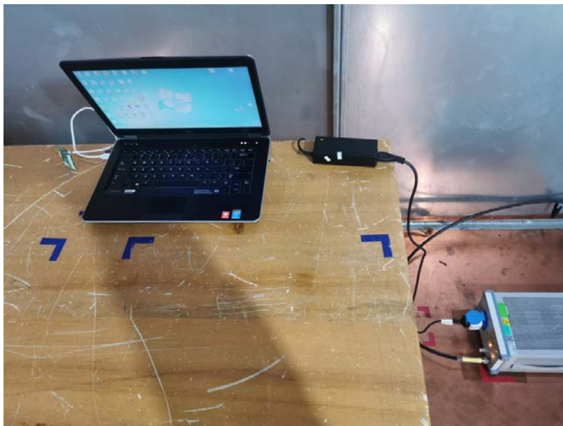
Conducted Emissions Test Setup (with charger)
