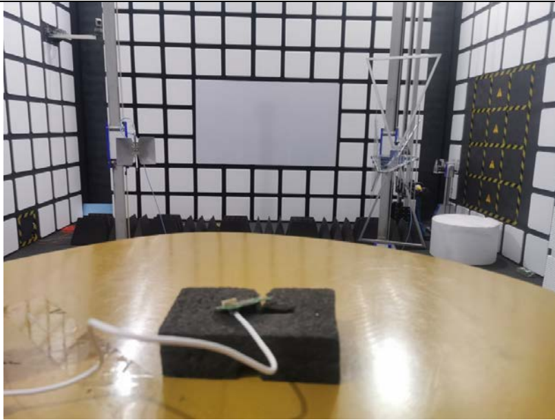
Spurious Radiated Emissions Test setup
