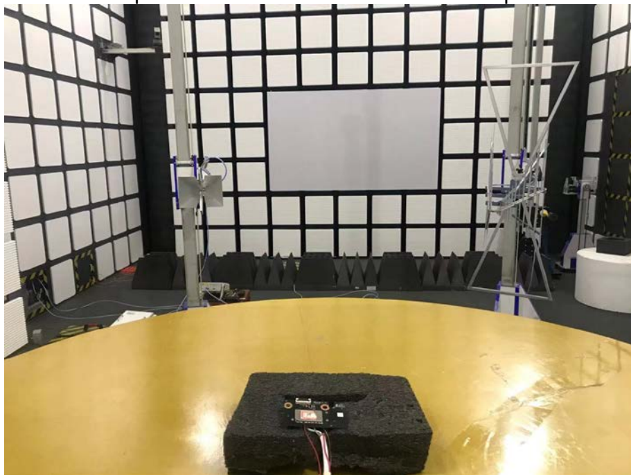
Spurious Radiated Emissions Test setup
