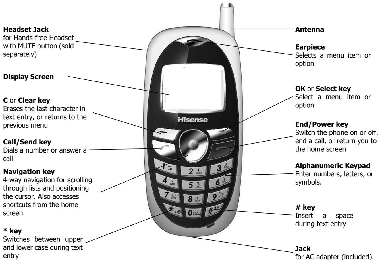
**Warning:** Inserting an accessory into the incorrect jack will damage the phone.
