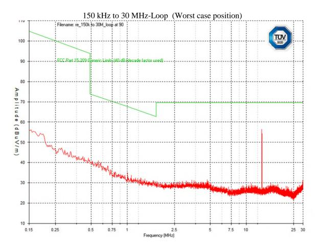
The worst case measurement as listed in the table below appeared at a Loop antenna position and a table azimuth as pictured in Appendix A.
