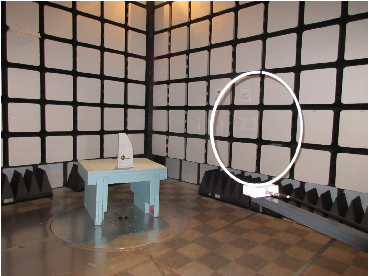
Figure 1 – Radiated Emissions Setup – Photo 1
