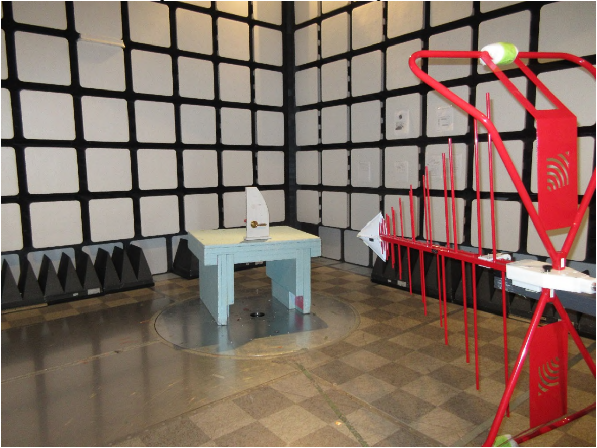
Figure 2 – Radiated Emissions Setup – Photo 2
