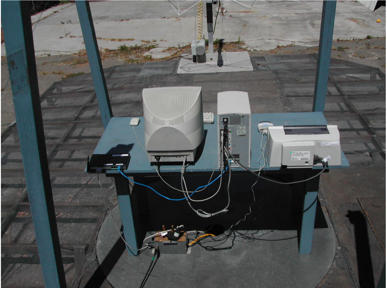
FIGURE 4: PLI Photograph Number 5405C2734SJ-03 the rear view of the Equipment Under Test in Conducted Electromagnetic Interference Test Configuration #1.
