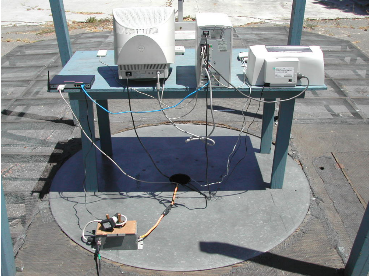
FIGURE 4: PLI Photograph Number 5405C2734SJR-01 the rear view of the Equipment Under Test in Conducted Electromagnetic Interference Test Configuration #1.
