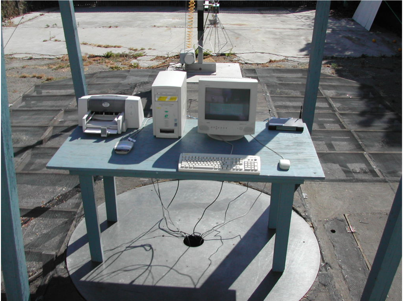
FIGURE 3: PLI Photograph Number 5405C2734SJ-01 illustrates the front view of the Equipment Under Test in Radiated Electromagnetic Interference Test Configuration #1.
