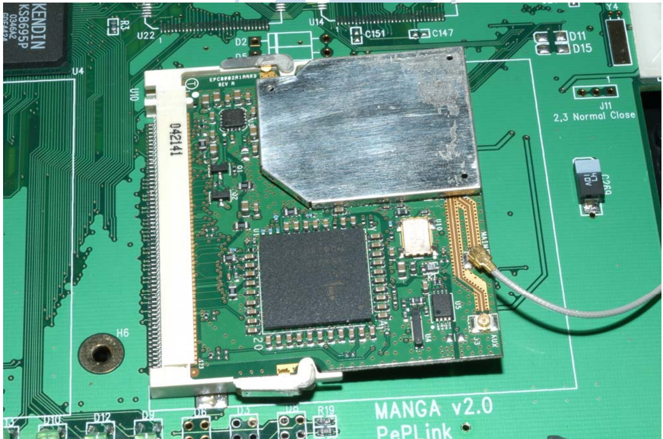
FIGURE 8: PLI Photograph Number 5405C2734LG-06 illustrates the information label removed from the transceiver printed circuit assembly installed on component side of the motherboard printed circuit assembly, MANGA v2.0.
