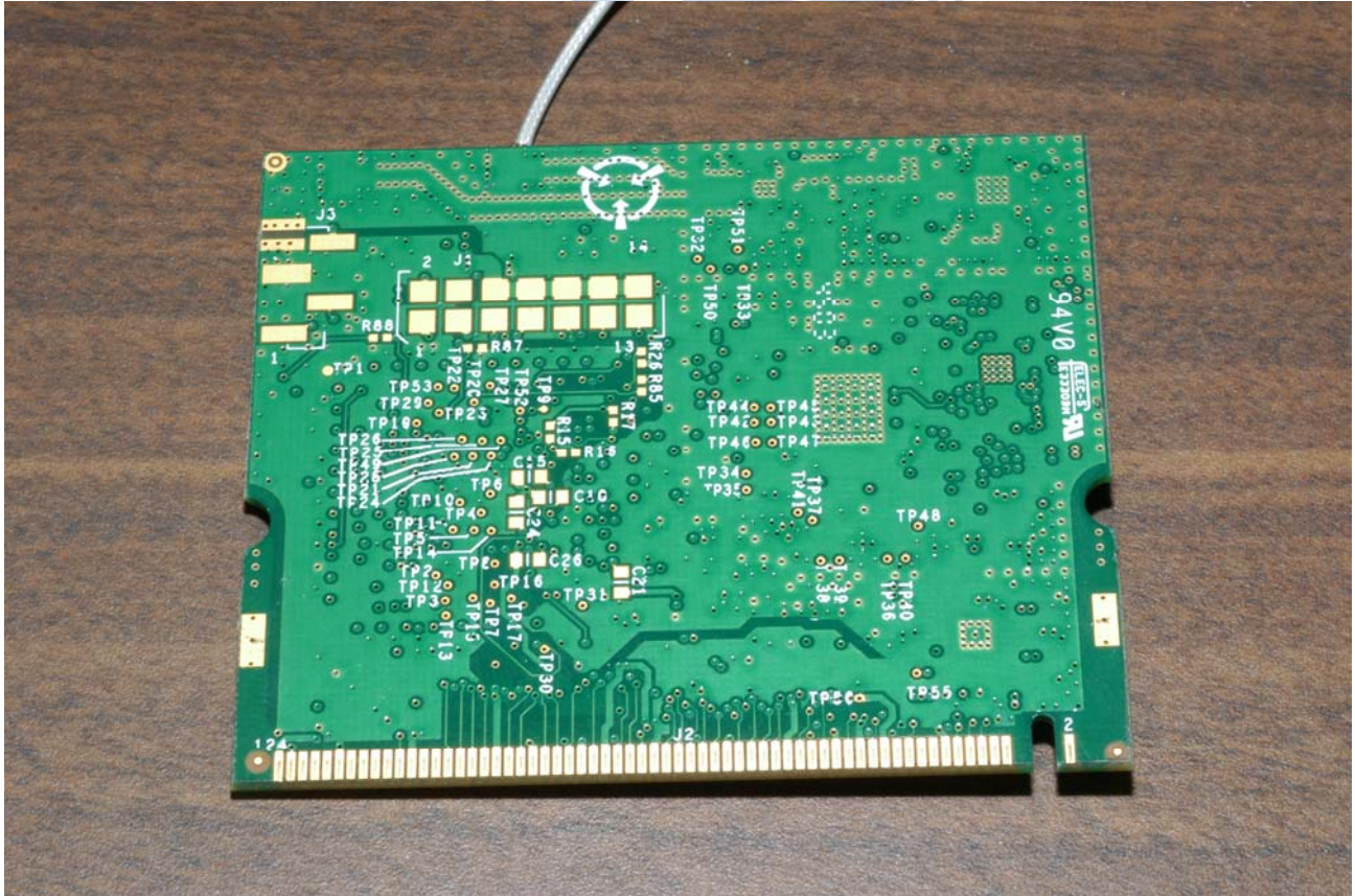
FIGURE 9: PLI Photograph Number 5405C2734LG-07 illustrates the circuit side of the transceiver printed circuit assembly uninstalled from the motherboard printed circuit assembly, MANGA v2.0.
