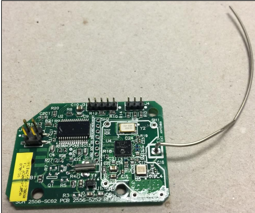
RF Module Top Side w/Shield Removed
