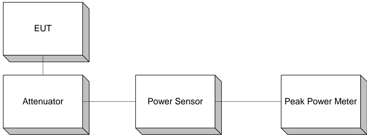
**Note:** A spectrum analyzer may be substituted for Peak Power Meter given that the measurement bandwidth is sufficient to capture the 6 dB bandwidth of the transmitter.
