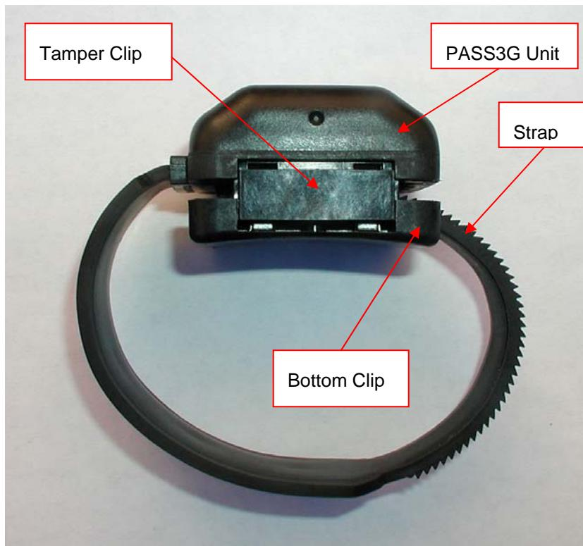
To install the PASS3G, first insert the two tamper clips (one on each side) into the main PASS3G unit housing as shown above. Next place the bottom clip partially onto the main housing until there is approximately a 1/8 inch gap (resistance will be felt). Place the unit on the wrist of the wearer and push the strap through the housing until it is snug. Snap the bottom clip onto the top housing so it is completely closed as shown below.
