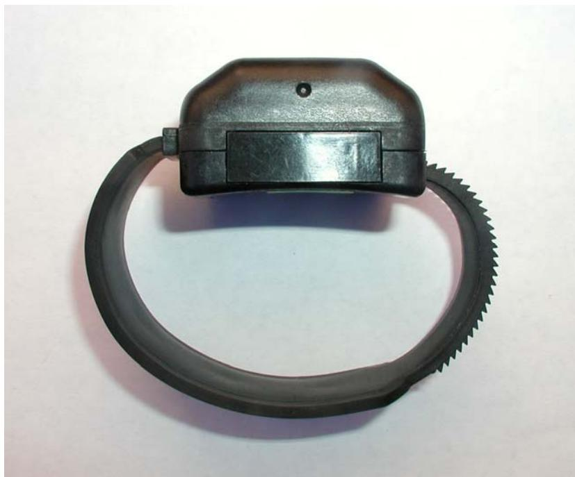
The PASS3G is activated via a wireless interface. This is done using the AeroScout Tag Manager application and the AeroScout Tag Activator.
