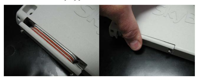
Ensure that the battery door is now firmly seated into the MT. Tighten the battery door/tray unit screws
