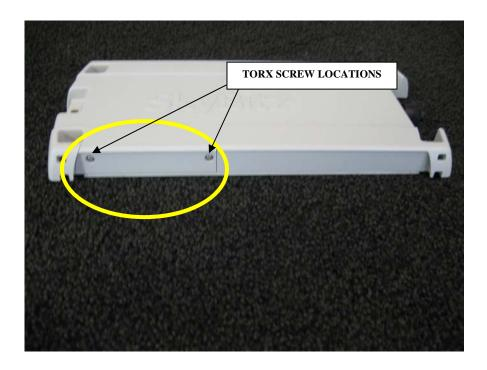
2. Using your fingers, carefully pull the battery door/tray unit out of the MT. This may be difficult due to the tight fit of the door and the dual O-ring seals. DO NOT ATTEMPT TO PRY THE DOOR AWAY FROM THE MT HOUSING USING A SCREWDRIVER or SIMILAR OBJECT. Set the battery door/tray aside being careful to keep the two "O" ring seals protected from dirt or other contaminants. Do not allow contaminants to get inside the MT through the battery access area.
