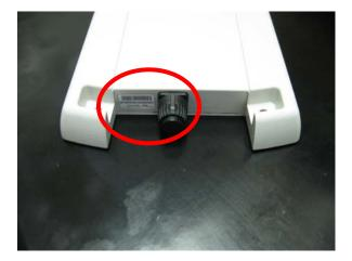
The fourth letter from the left indicates the REV type. For example the serial number on a SkyBitz REV M mobile terminal will look like "MTXM3GDLxyyyzzzzz", where "xyyzzzzz" are numbers. The "M" after "MTX" indicates the mobile terminal REV type. The serial number on a SkyBitz REV P mobile terminal will look like "MTXP3GDLxyyyzzzzz", where "xyyyzzzzz" are numbers. The "P" after "MTX" indicates the mobile terminal REV type.
