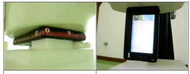
The bottom of the EUT face to the phantom with 0mm-separation distance.
