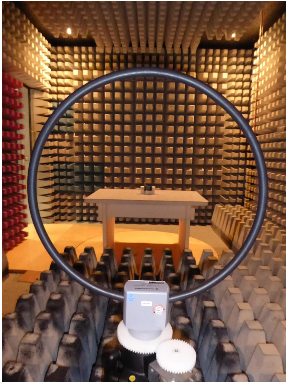
162386_20.JPG: WM2.4, test set-up fully anechoic chamber
