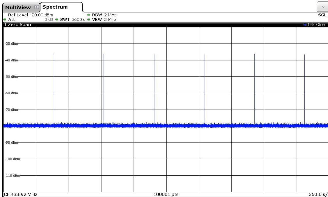
162386\_1h\_zoom1burst.png: Total transmissions in one hour with zoom to one burst packet:
