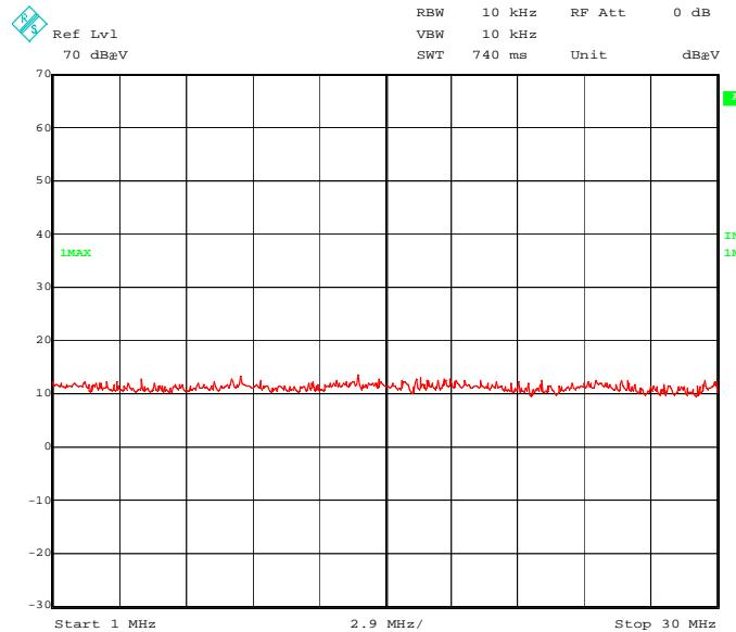
No frequencies were found during the preliminary measurement, so no final measurement on the outdoor test site was carried out.
