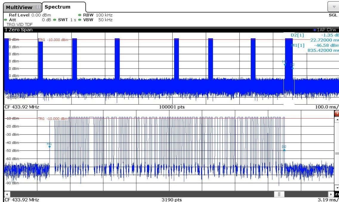
Measurement of the total transmission time per hour:
