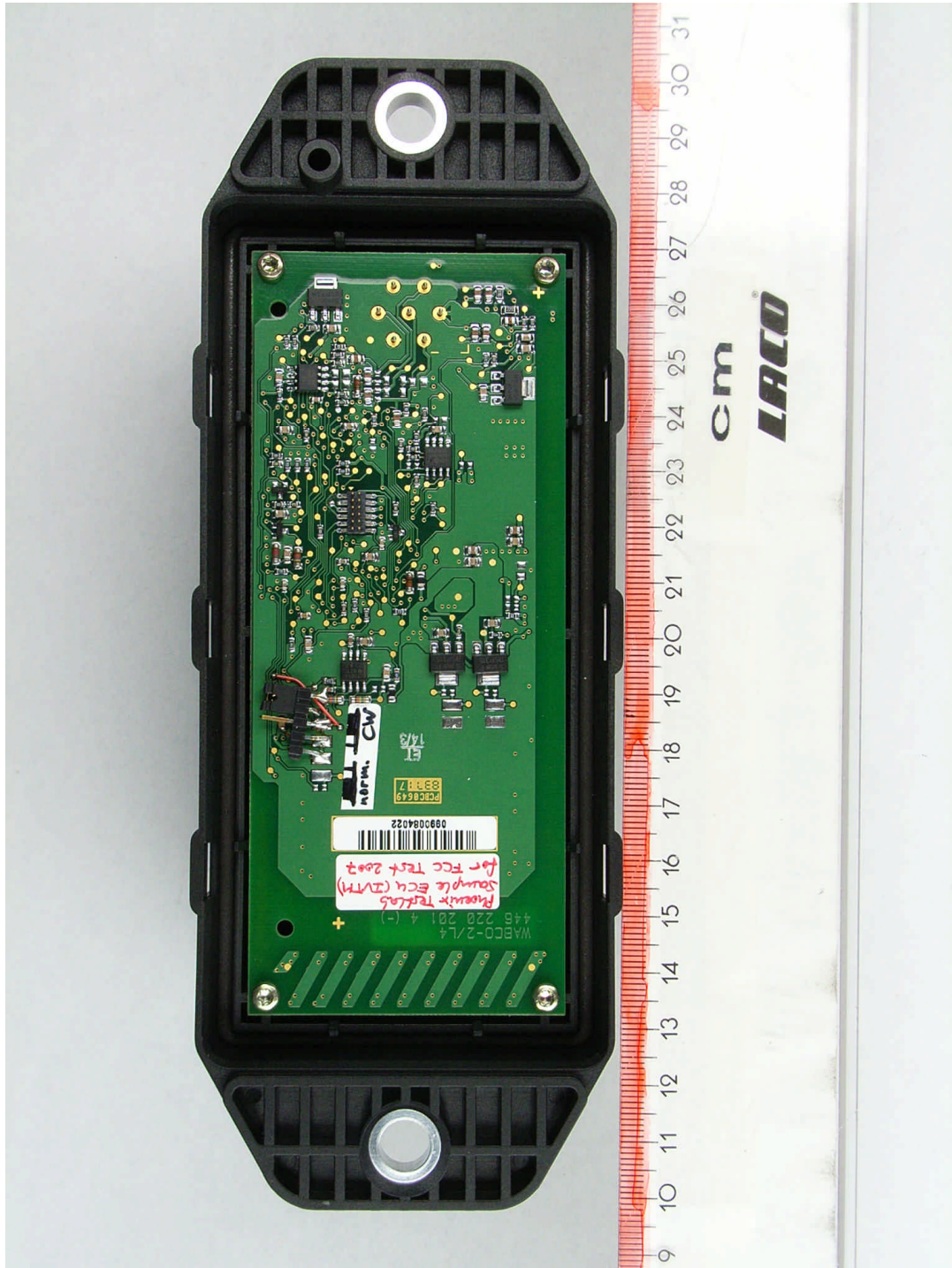
71209eut4.JPG IVTM ECU, enclosure opened
