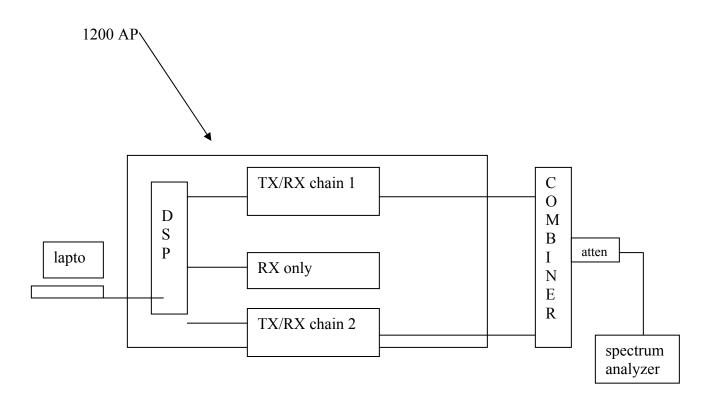
3. Please provide peak output power measurement data for the following mode of operation:
