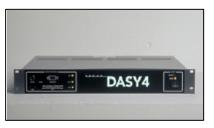
The DASY4 measurement server is based on a PC/104 CPU board with a 166MHz low-power Pentium, 32MB chip disk and 64MB RAM. The necessary circuits for communication with either the DAE3 electronic box as well as the 16-bit AD-converter system for optical detection and digital I/O interface are contained on the DASY4 I/O-board, which is directly connected to the PC/104 bus of the CPU board.
